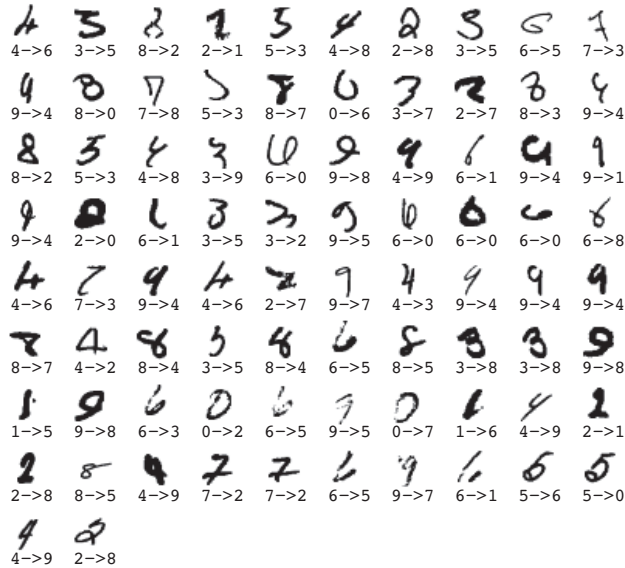
Figure 16.15 These are the 82 errors made by LeNet5 on the 10,000 test cases of MNIST. Below each image is a label of the form correct-label \rightarrow estimated-label. Source: Figure 8 of (LeCun et al. 1998). Used with kind permission of Yann LeCun. (Compare to Figure 28.4(b) which shows the results of a deep generative model.)
